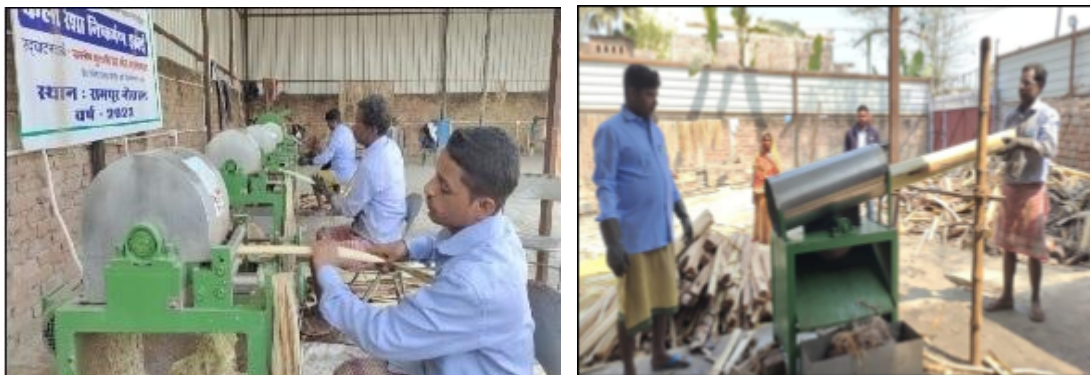
Fig. Cutting and Fiber extraction of Banana Pseudo stem
