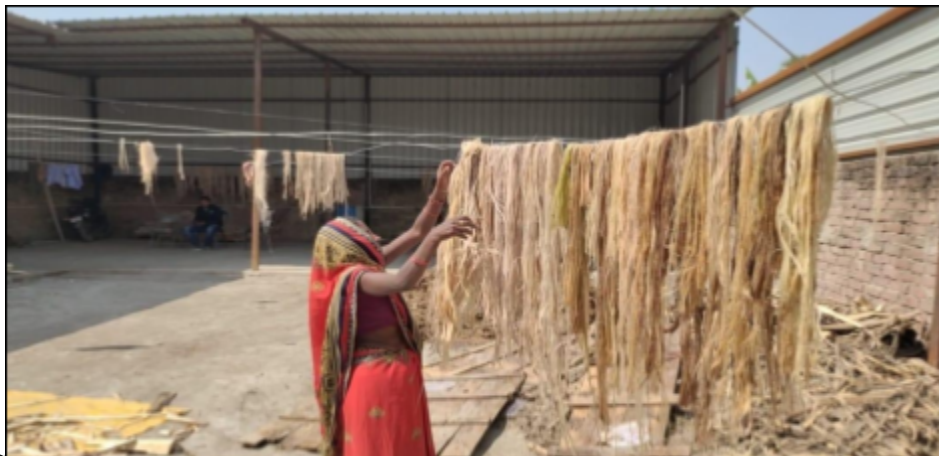
Fig. Drying of extracted raw banana fiber
